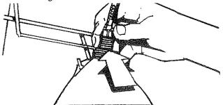
Slide the adjustable nozzle forward to low pressure mode. Detergent cannot be applied with nozzle in high pressure position.
