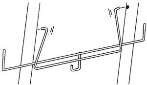
• Cut tie wrap on chemical injection tube. Remove chemical injection filter, thread chemical injection tube through the wire form and reinsert filter into tube.
