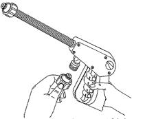
• Remove plastic cap and connect high pressure hose to pump. Tighten by hand.
