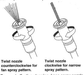
For most effective cleaning, keep spray nozzle between 8 to 24 inches away from cleaning surface.
